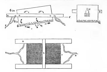
Figs. 1, 2, 7.—Green's patent hatching box seen from the side, end and bottom. Scale, 1-20th. a. side floats 3.4" long; 2" by 3" square, set with screws. b, bottom cross bar, bevelled, to throw the current upward. c, wire-net bottom 14 wires to an inch. d, trap in hind end for escape of young fish, covered by wire-net, 8 to an inch, and with a covering slide. e, anchoring cord. f, water-line. G, spawn.
