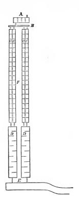
sent the flannel screens; if there were four it would be better. The water entering the first apartment on the right, passes through the screens and flows into the distributing trough B, which by four jets supplies the troughs  $c \ c \ c \ c$ .
