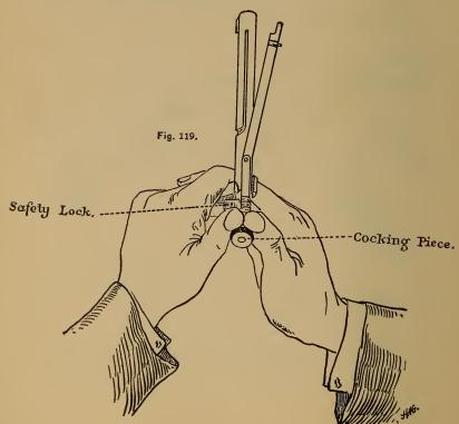
4. Grasp bolt and cocking piece as in third operation for dismounting. Draw back and turn cocking piece from the operator until its nose enters the notch on the rear end of the bolt (see Fig. 118).
