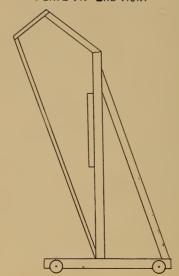
wheels or casters that it may be moved and used in any desirable position in the room. The protection shield for the lights is made part of the framework. See plate A.
