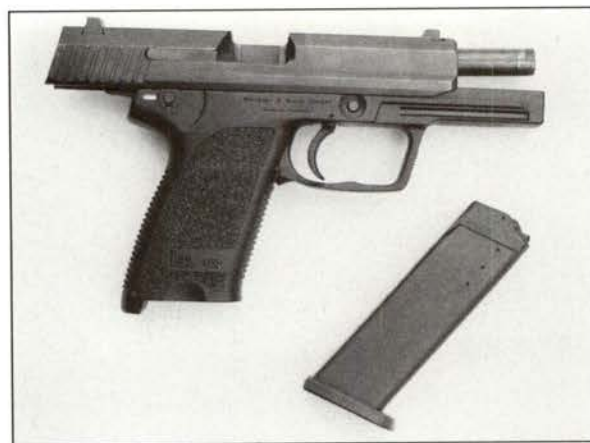
Top: Heckler & Koch USP (Universal Self-loading Pistol), 9mm double stacked pistol. The large catch at the rear is the safety catch when pushed up and the de-cock lever when pushed down—the sort of safety the Browning BDM should have! Above: Heckler & Koch 9mm pistol with the slide locked open. Note that the barrel tips slightly, as invented for Colt by John Browning early in the twentieth century.
