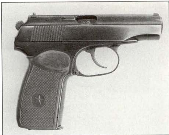
Above left: 9mm Makarov service pistol, right side—a straight derivative of the Walther PP. Note the small ejector port.
