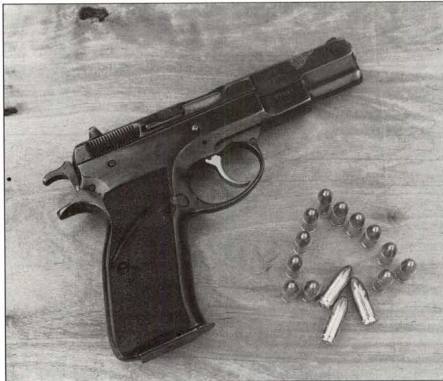
Left: 9mm CZ75, a 15-shot double-stacked auto pistol with features derived from both the Browning Hi-Power and the SIG P210 pistols. Introduced in 1975, it anticipated the trend towards high-capacity auto pistols. Above right: Beretta 92FS with the slide removed. The barrel does not tip towards the magazine as do Browning designs, but the magazine presents the next round high enough for virtually straight delivery into the chamber. Above far right: SIG P226 9mm pistol, the only serious rival to the Beretta 92F in the (some say fixed) US adoption race.
