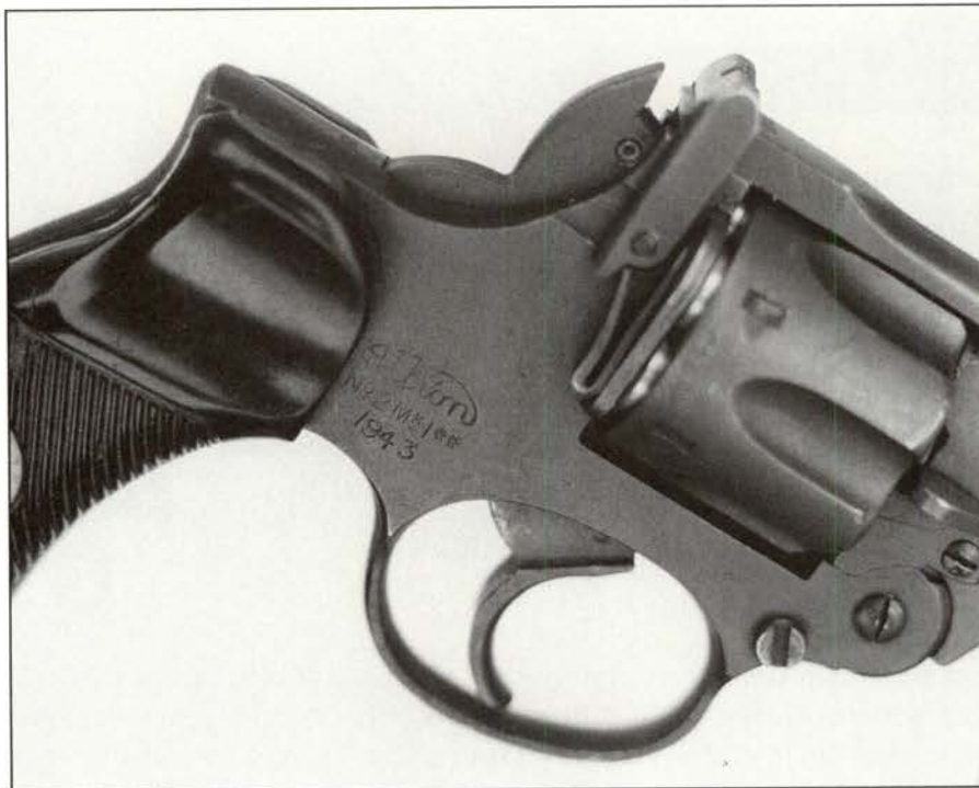
Left: Close-up of No 2 Mk 1** revolver, showing the Albion logo and year of manufacture (1942). The first star denotes double action only, as seen from the absence on the hammer of a cocking spur, and the second star denotes a safety stop, left out of later production models to speed manufacture. Double star models can go off if dropped on the muzzle! Note black bakelite grips with finger extensions: we have also seen this pattern of grip made in walnut and white metal.
