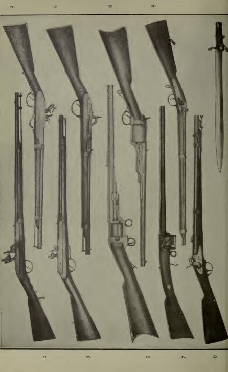
length of barrel 21 inches; calibre .54. The hook-shaped catch for the preceding pattern having not only proved inconvenient for the cavalryman but also capable of inflicting troublesome wounds, a remedy was sought in this device.
