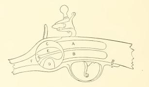
These compartments connect by cylindrical passages with the central chamber in the frame, in which is located a solid cylindrical block (c) with its axis from right to left.
