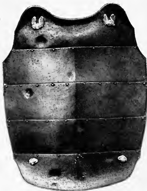
Fig. 129. Japanese breastplate with marks of bullets, 1750 ?
