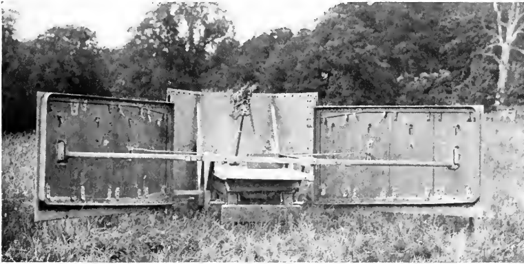
Fig. 142. Mobile shield or "pedrail" for machine gunner and riflemen. British model, 1917
