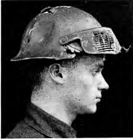
Fig. 43D. Polack visor with new experimental French helmet (1918). Die stamped. Specimen tested in H. A. E. F.
