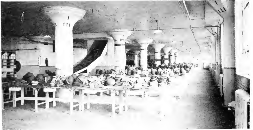
Fig. 157. British-American helmet. Assembling. Helmet shells being passed down an inclined plane to tables where linings and chin-straps are put in place
