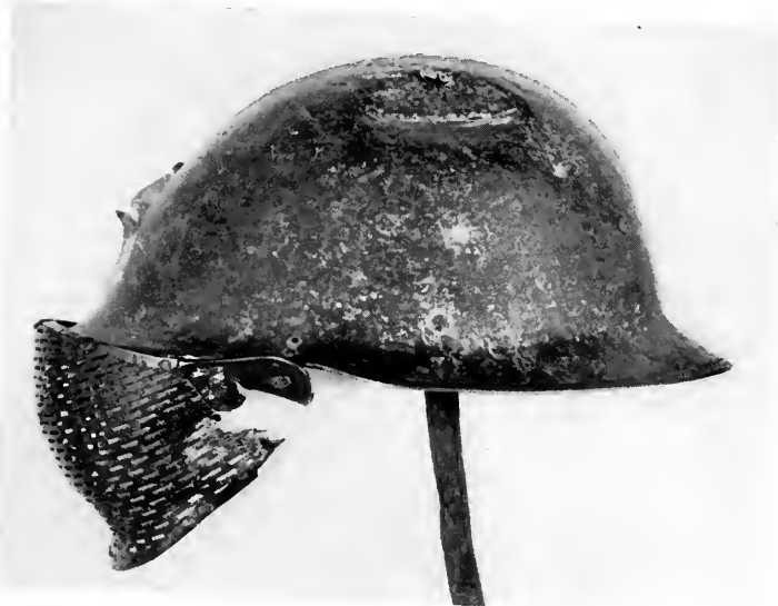
Fig. 48. Dunand helmet, showing result of tests
