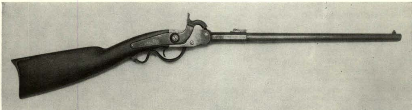
Again marked UNION RIFLE this Cosmopolitan No. 4, last type, has improved carbine rear sight and flat hammer adapted for machining. Lever screw is larger head, from right of breech. Lever has improved rear end catch.
