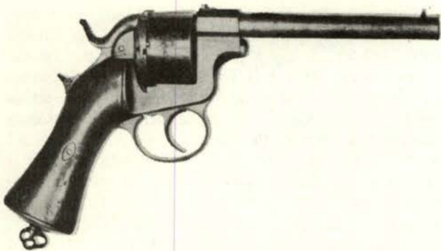
Open-top "Raphael" revolver may be one of 106 actually purchased from George Raphael in New York. Maker or inventor of design is unknown but gun used special centralfire inside primed cartridge, and was double action.
