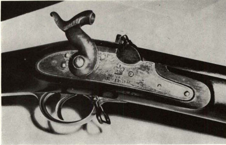
Crisp lock fitting is seen about cone seat of early percussion British sea service musketoon. Gun is model arm transformed from flint, was in Liege gunmakers' museum as a sample for many years. Huse bought similar guns.
