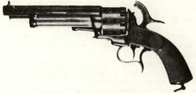
First Model LeMat carried by General P. G. T. Beauregard has "cavalry" spur guard and compound loading lever on right side of half-round barrel. Hammer nose has tiny studs on sides of movable tip. Barrel latch is pivoted in frame above trigger guard base.
