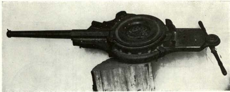
Repeating turret magazine cannon of small bore and considerable ingenuity is credited to invention of Confederate Ordnance General Josiah Gorgas. South used several repeaters and rapid fire breech-loading Williams gun also.
