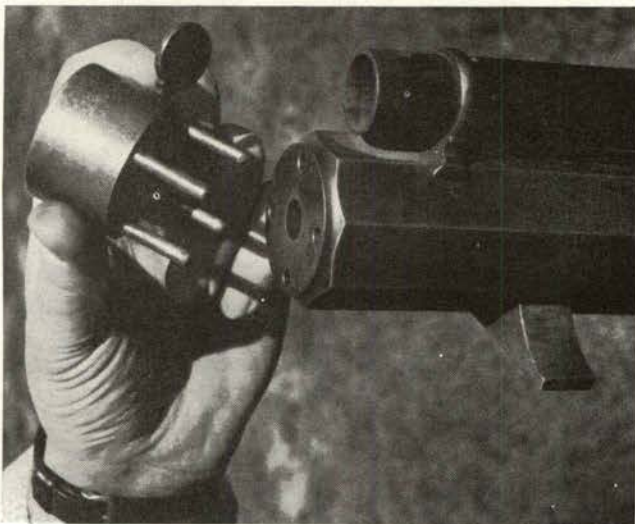
False muzzle is put on, to protect end of rifling from ramrod wear and deliver bullet from muzzle with greatest precision. Thumb-blade is to obscure vision through scope when muzzle piece is installed so accidental shot will not throw it down range and damage rifle.
