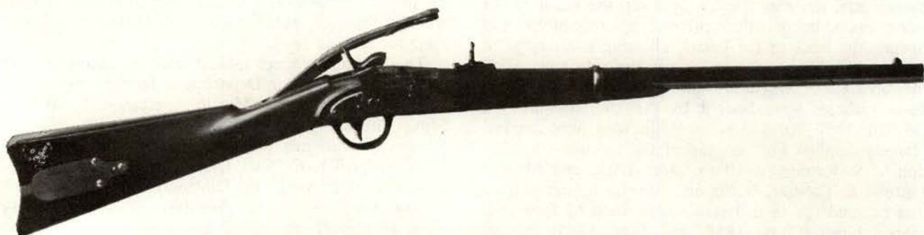
Production Merrill carbine had top lever latched at front end to rear sight fixed base. Raising lever pulled back toggle plug in barrel for loading with combustible cartridge. Second type omitted patchbox, changed shape of lever latch piece to round nuts from elaborate filed contours of first type.
