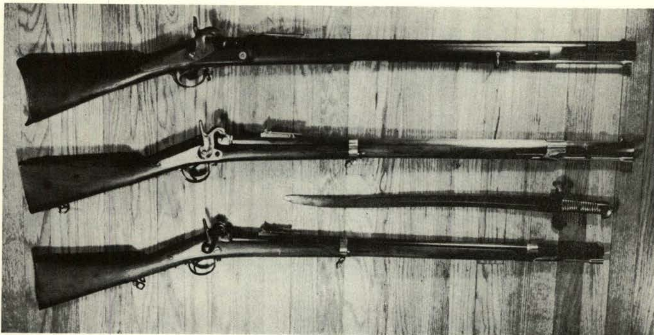
Among best arms bought abroad were Thouvenin system rifles from Dresden, a heavy but accurate .69 round ball gun (top); and French minies. Thouvenin rifle is steel trim, casehardened with blued barrel; Carabine de Chasseurs de Vincennes (middle) is bright with 4-groove .69 bore for minie bullet. At bottom is elegant .58 "beautiful minie," brass trim, blued, weighing 7½ pounds.
