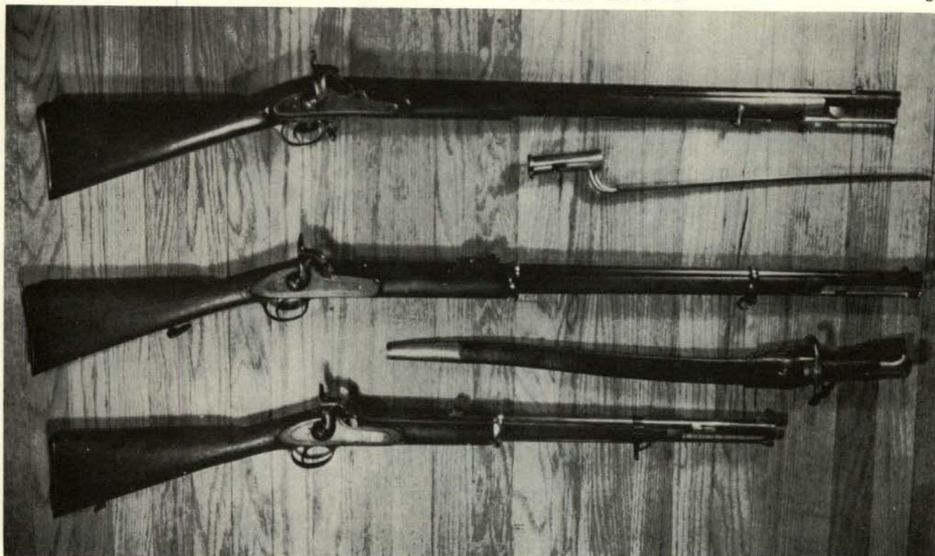
Accenting finest available for the money, Southern buyer Huse took best of older British muskets (short sea-service shown top, and detail) and best Enfields. Hand-made Pryse & Redman, middle, is 1859 sergeant's rifle, has unmarked lock. Bottom is Enfield carbine engraved London Armoury Co. with Southern-association JS-Anchor stock stamp. Carbine was found in Tennessee. Both Enfields take sword bayonet with iron-trimmed leather scabbard.
