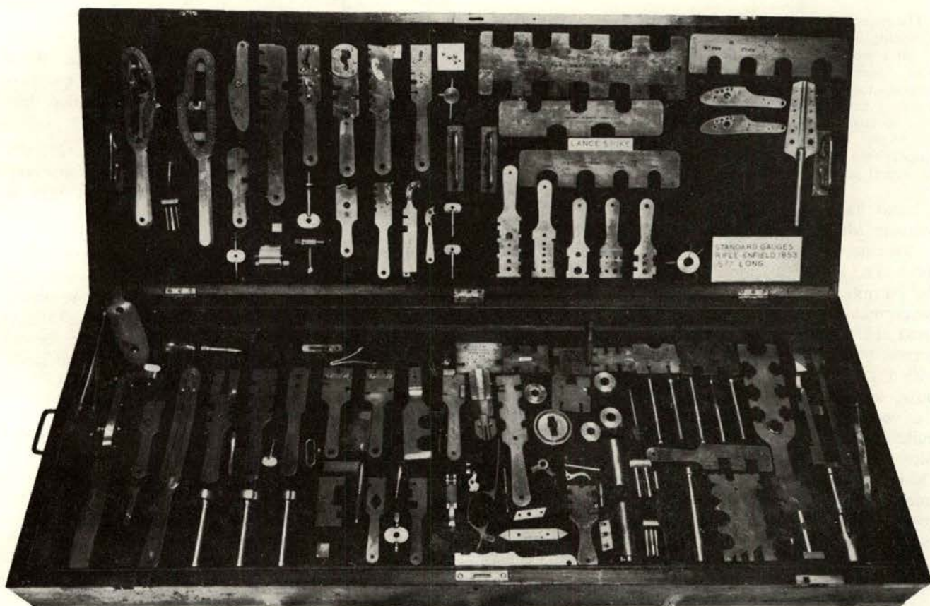
Extensive gauging was to be introduced in South's production scheme by Macon Enfield factory. Gauge set shown is from Enfield Armory.
