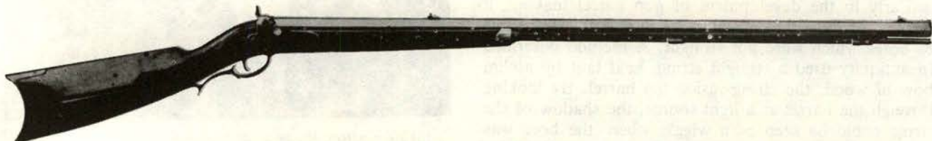
"First rifle" often pictured in Remington literature is actually percussion half-stock American sporter of 1840's and was made several decades after Eli Jr. founded gun firm. Cheekpiece on right as well as left of stock is sometimes found on Remington-built early rifles.
