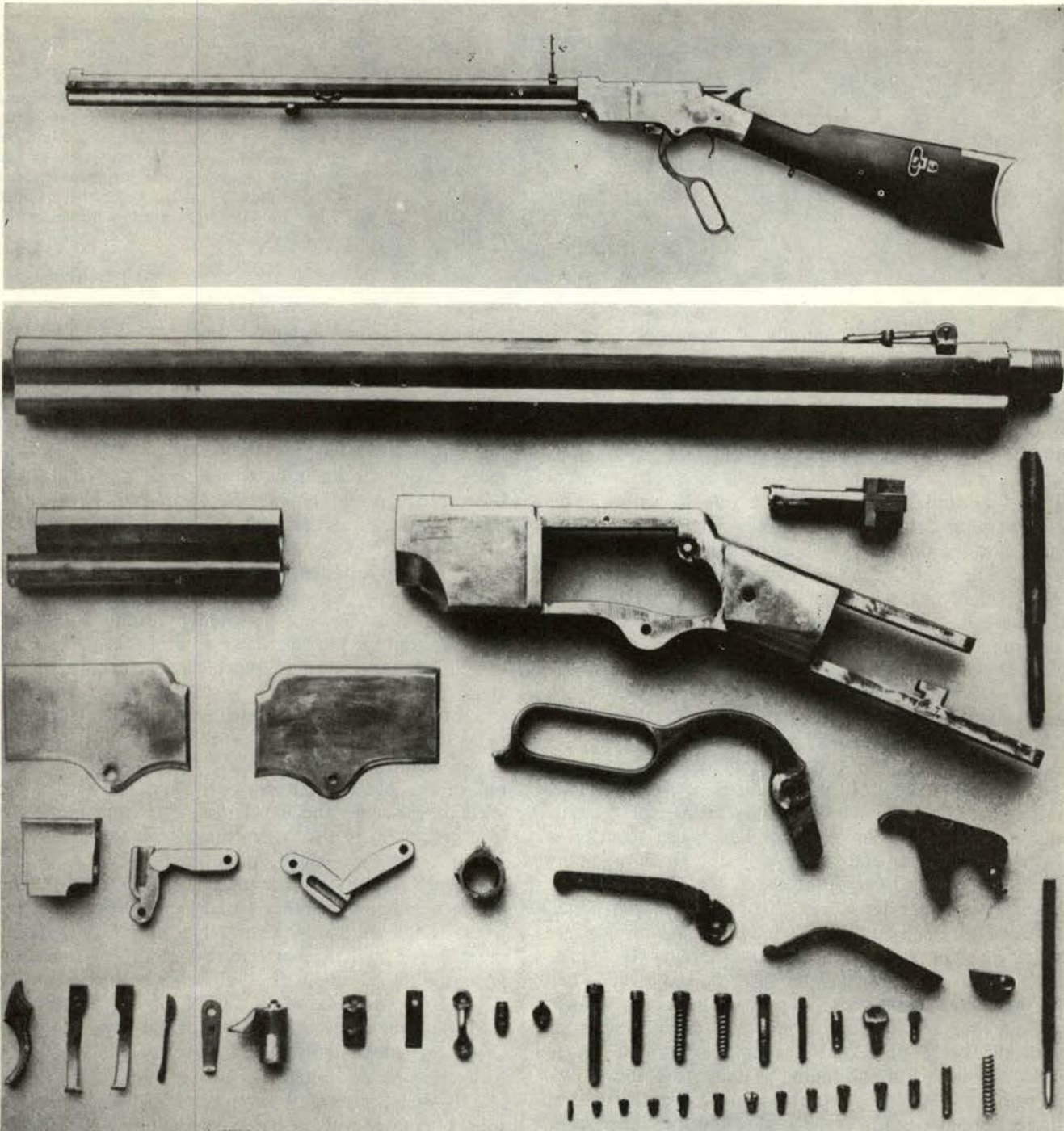
US Government test report of Henry rifle pictured gun complete, showing lever in down position and breech bolt withdrawn which cocked gun, and also all parts. Double pieces near lower left of disassembled view are toggle links that collapse when lever is moved. Principle is identical to enigmatic Italian Vendetti pistol, suggesting missing link which designer Horace Smith found overseas.
