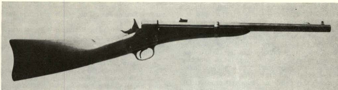
Split-breech carbine is shown with block partially rolled back. Arm was contracted for by Sam Norris but not actually delivered until after war. With Rider's improvements, design became famous Remington Rolling Block single shot.
