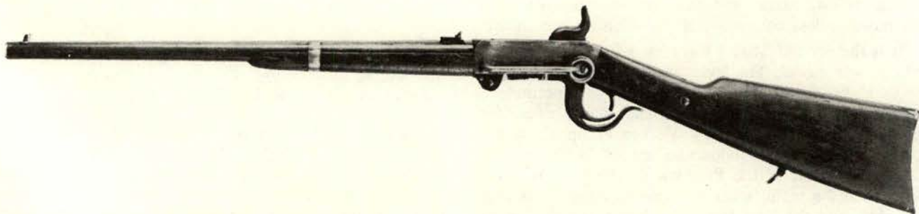
Fourth model carbine had Foster's improved lever, and barrel band held by spring on under side of stock. In fifth type, side screws were added in breech box to guide motion of receiver, which had corresponding cam cuts in its sides.
