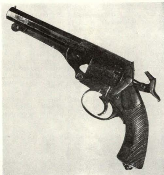
Often assumed to be double action guns that don't work. Kerrs are usually single action with a trigger that moves to rear of guard for creepless let-off. Caliber is .450 but .36 Kerrs are known. Some were made in Liege.
