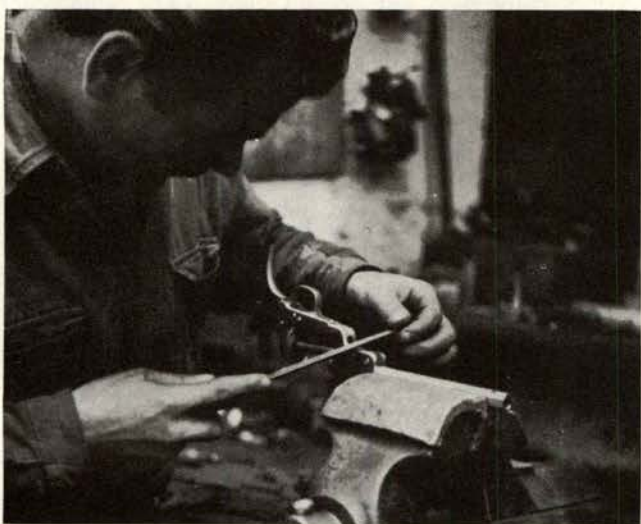
In Brescian shop of Vittorio Gregorelli fine Italian hands put together copies of Colt Navy revolvers. Workman standing takes whisker of metal off brass "Reb" backstrap while man with file shapes curve of 1851 barrel frame.
