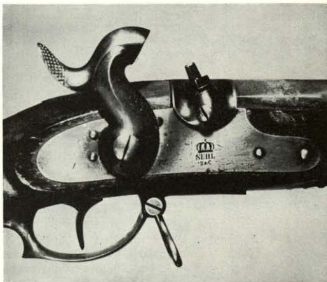
Superior Prussian muskets were the Model 1839, shown here with locks of Zella (twin cities Zella-Mehlis are gunmaking towns) and Suhl. Cone seat is patent breech that unscrews from barrel. Guns were surplus in 1861 because of German states' rearming with new "needle gun" breechloader.
