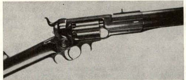
In 1857 about 300 cal. .44 revolving rifles had been bought for field trial issue; specimen shown has hooks to place supporting hand in firing. Inspection stamp of William A. Thornton, WAT , is on side of stock.
