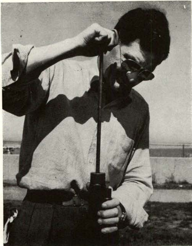
Bullet is seated firmly but not heavily on powder by brisk motion of stiff bore-fitting ramrod. Hickory is used for ramrod to avoid damaging rifling as barrels were iron or soft steel.
