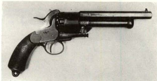
Paris-finished Navy Second Model LeMat No. 1666 in M. Clifford Young, Boston, collection, has screw-barrel latch of simple form with spring on side attached to barrel. Hammer nose has tail through hammer head slot.
