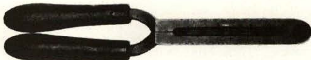
Six-cavity Sharps rifle or carbine mould cast .52 cal. conical bullets but user had to trim excess lead off bases.
