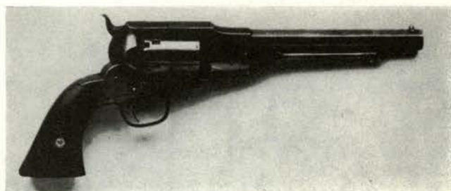
Beals type pistol is distinguished by frame covering back of barrel and square shank of loading lever. Arm was sold to Union in .36 and .44 sizes, identical in design but differing in size.
