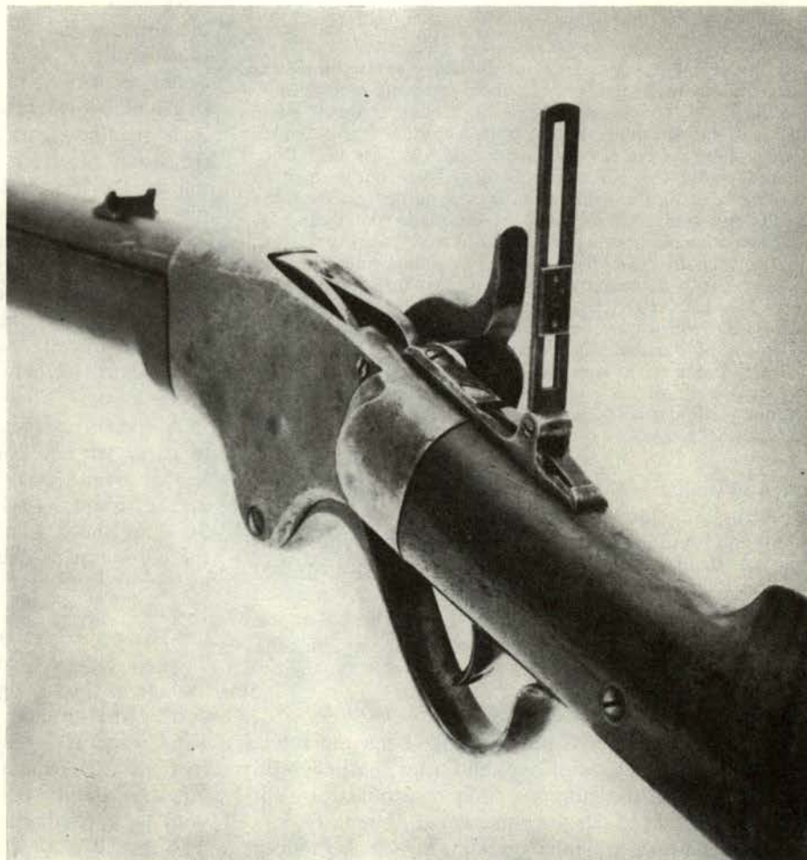
Special Spencer sporting rear sight is unique pattern with these rare arms, does not have large disc peep so characteristic of sights of following decade. Gun is listed in 1866 catalog but is believed to date from early in the war. Flange on butt plate is end of loading tube which, turned aside, is pulled out to insert seven cartridges into magazine. Design was heavy, but foolproof. The loading tube (not shown) is carried in a recess in the stock, and inserted through the butt plate.
