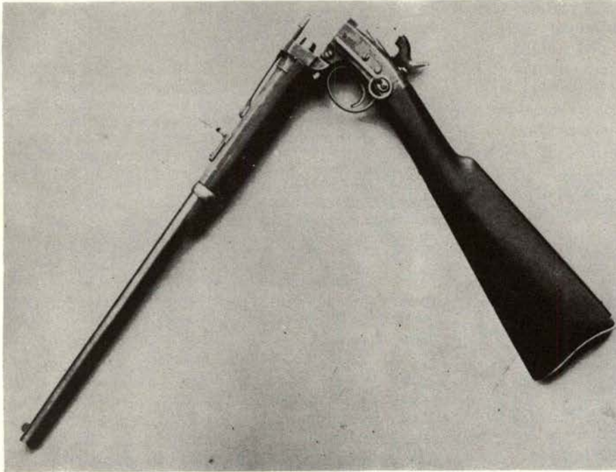
Hinged breech was feature of Gilbert Smith's carbines made by Mass. Arms, American Machine Works of Springfield and American Arms of Chicopee Falls, for Poultney & Trimble of Baltimore who contracted for them with the Government.
