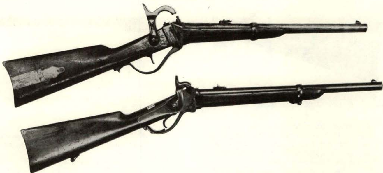
At Enfield Armory, Burton in late 1850s supervised modification of Sharps carbine to placement of nipple directly on barrel; then actually made at least two Sharps Carbines at Enfield, one of which shown has cone flashing into chamber without complicated channels in breech block. Experience was drawn upon by Burton in setting up Richmond factory.
