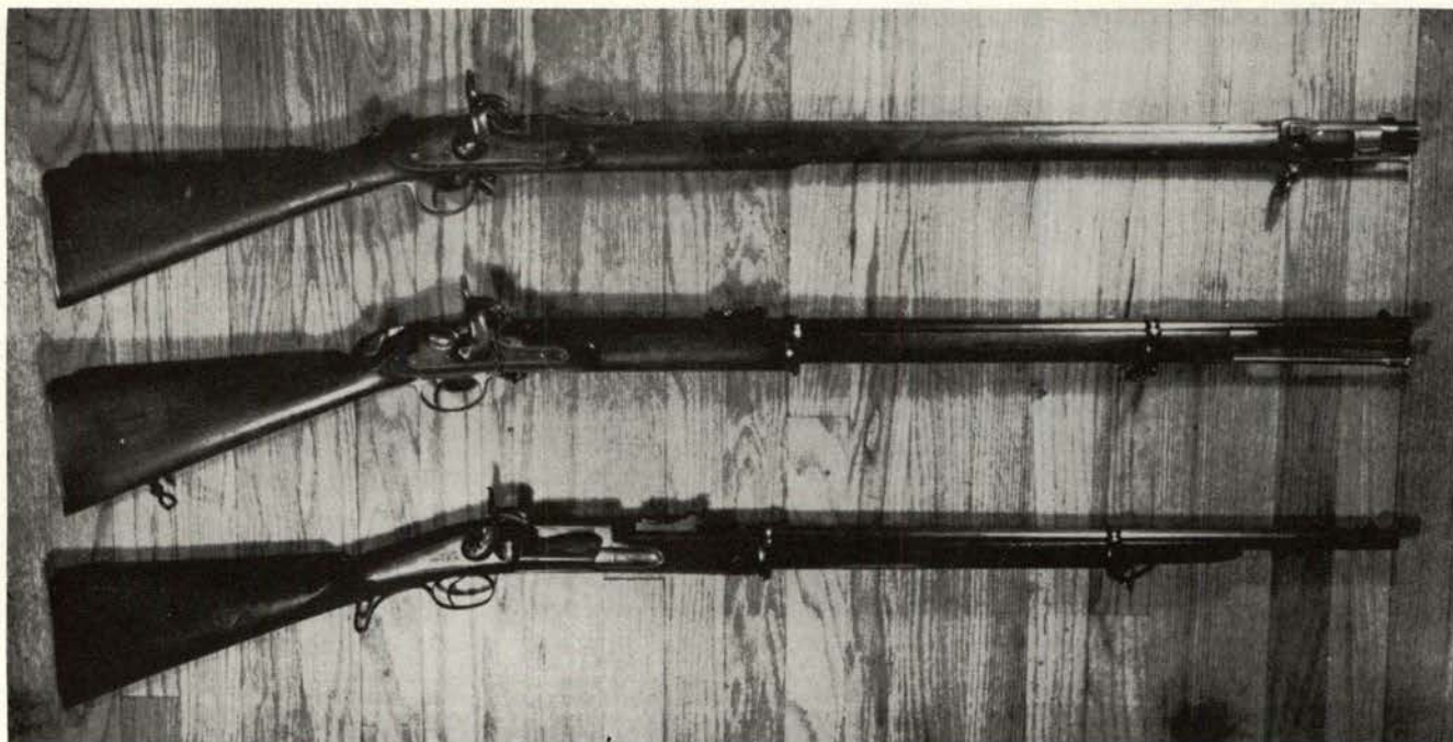
Alleged breechloading Civil War rifles are (top) Westley Richards M1860, .450 Whitworth caliber, with bayonet stud on front band; Wilson's sea-service or sergeant's rifle with bayonet stud on barrel, and, bottom, "Breechloading Gun Co." .577 Leetch patent short rifle with side-swing block. Bayonet stud resembles that for Sharps, Spencer rifles.
