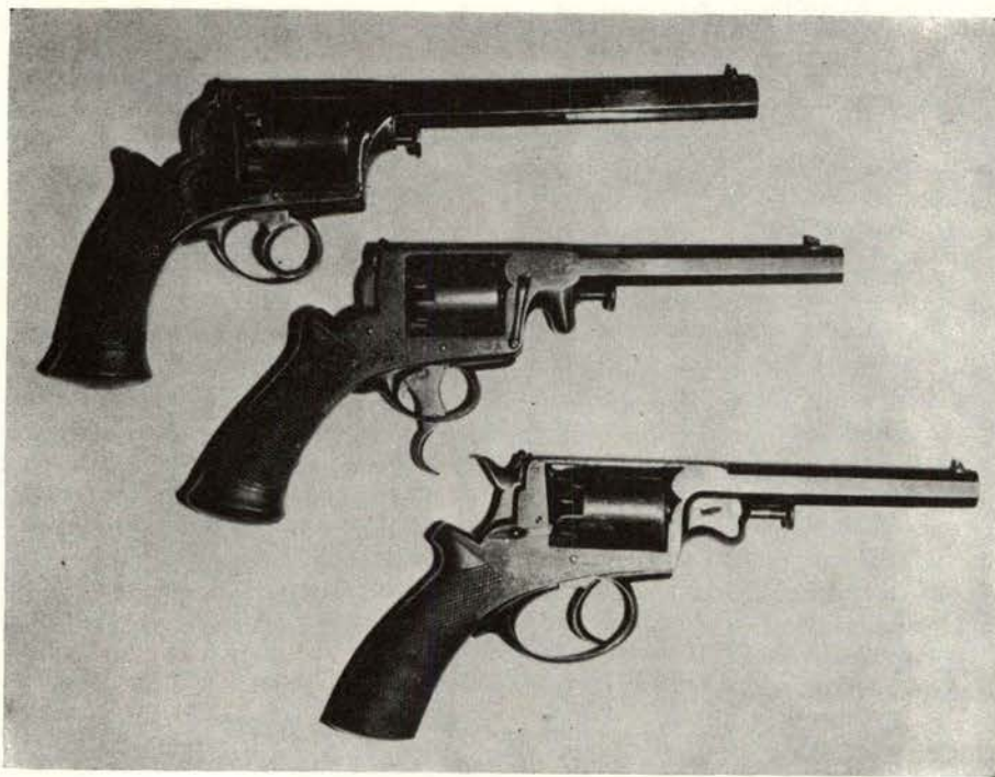
Hartley became agent for London Armoury Company's Adams revolvers in New York, sold small quantities to U.S. buyers. Top is big 1851 DA Dragoon .50; middle is Adams with Tranter's patent double trigger made by licensee August Francotte; bottom is Beaumont Adams 1856 .450. Same model was also made in U.S. by Mass. Arms.
