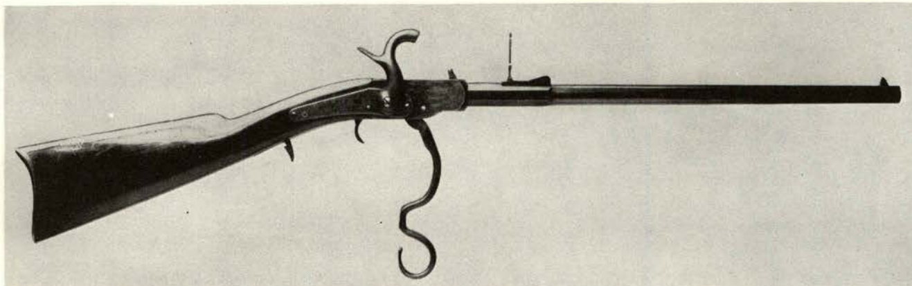
Cosmopolitan No. 3, First type, has same round hammer but breech is Gwyn and Campbell patent though old company name with Gross Patent is still stamped on lock. Lever screw enters from left of breech box. Not marked UNION RIFLE.
