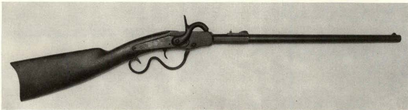
Cosmopolitan No. 3, Second Type, has lever screw from right of frame, and new Gwyn & Campbell mark is stamped on lock. Lever curve does not meet tang of trigger plate on this variation. Gun is rusty but not marked UNION RIFLE.
