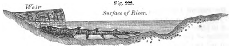
MINUTE OF A TREE IN THE PROTECTION OF RIVER-BANKS.
