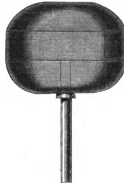
VIEW OF CARBON FILTER.
