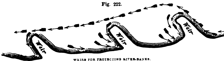
WEIRS FOR PROTECTING RIVER-BANKS.
