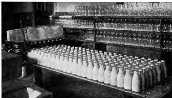
FIG. 219.—Milk bottled for the retail market. The machine at the left fills eight bottles at once and is then moved to the next row.
