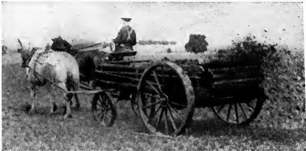
FIG. 46.—A manure spreader at work. This machine can be regulated to spread the manure thick or thin on the field. The spreader makes the best use of the manure, saves labor, and produces the most uniform crop.
