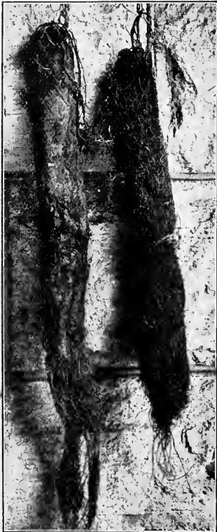
FIG. 13. Photograph showing willow roots as taken from a tile drain which they had completely clogged. (Edgerton.)
