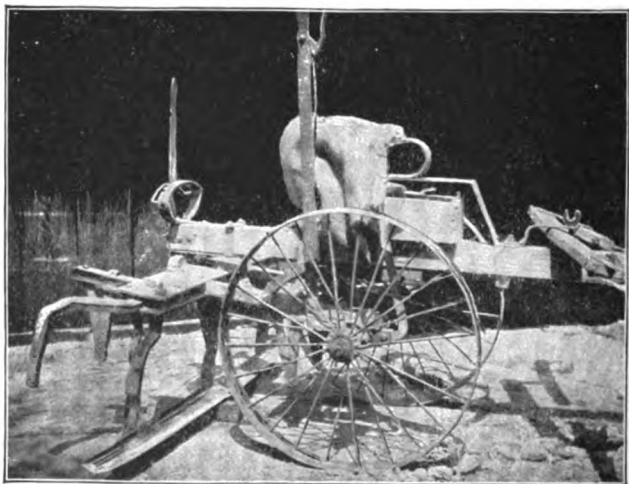
Fig. 111. Combined orchard cultivator and furrowing tool.
