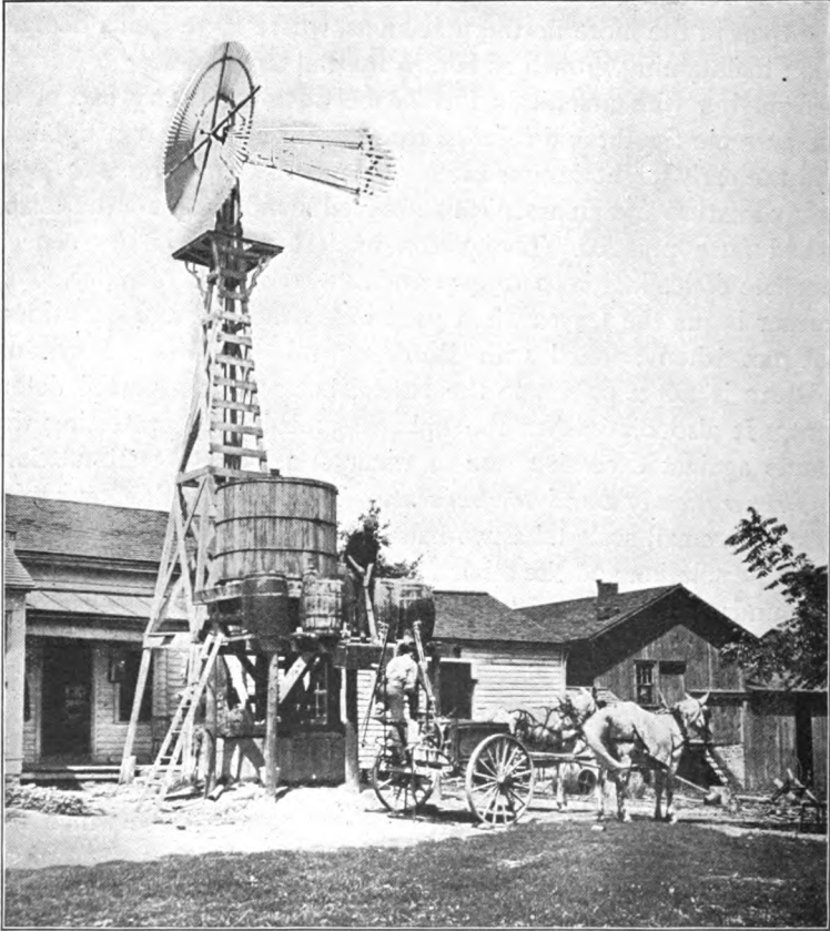
FIG. 129. Equipment for making Bordeaux mixture — tank, stock solution and dilution barrels, and power sprayer
