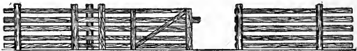
Figure 64.—Farm Gate Intended for Grain Fields and Pasture Fields at a Distance from the Farm Buildings
