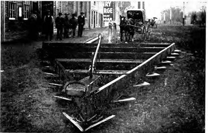
THE BATES GRUBBER FOR CLEARING SAGE-BRUSH Pulled with 35 H. P. Engine
