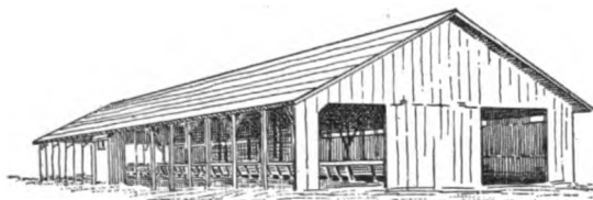
Fig. 186. Shed for hay feeding, showing simple construction. The feed-racks run lengthwise through the center.
