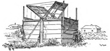
Fig. 266. Jumbo or paddle-wheel mill which rotates in the same plane as the wind.
