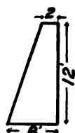
Fig. 403. Cross-section of a rough stone or concrete dam that may be used in gullies, the sides and bottoms of which are of rock.
