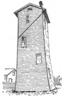
Fig. 415. A housed-in tank. The inclosed space may be used for a tool-room. In cold weather a fire may be kept to prevent freezing.
