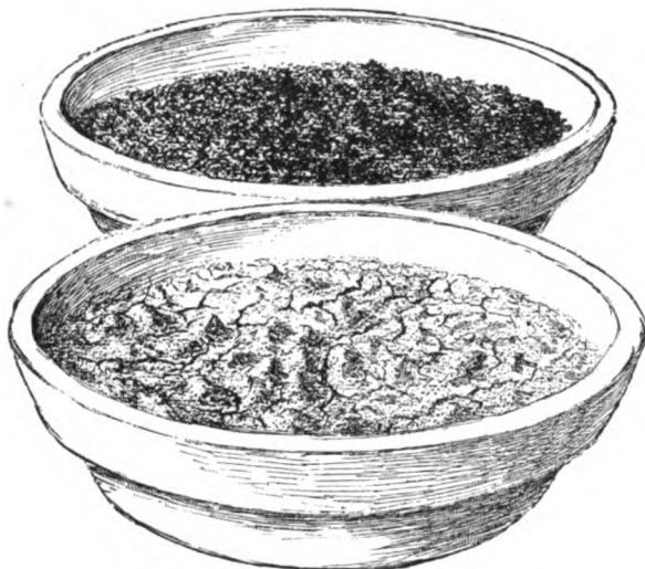
Fig. 476. The texture of the soil. The upper sample is loose garden loam. The lower is hard pulverized clay. Both were given the same quantity of water and allowed to dry. The loam remains loose and crumbly; the clay puddles and cracks.
