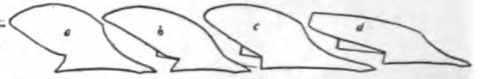
Fig. 512. Characteristic styles of plow bottoms. The types vary from the long, sloping share and moldboard of the breaker plow (on the right) to the short, abrupt curvature of the old ground or stubble plow (on the left). The intermediate forms are for "general purpose" plows.
