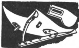
Fig. 517. Heel plate, used to vary the width of surface at the heel.
