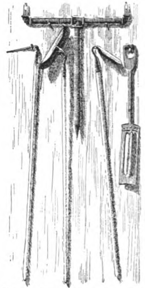
Fig. 578. Draining tools. A simple home-made form of water-level at the top, made of iron pipe with water-gauge glass in the elbows at the ends.
