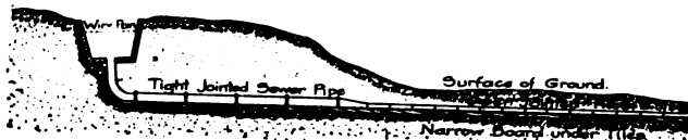
Fig. 411. Methods of receiving and discharging sewage. In this section, the sewage passes continually from the receiving tank into the drain pipes. In Fig. 409, which is the better, the discharge is intermittent.
