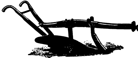
Fig. 496. Type of sod plow, which pulverizes but little.
