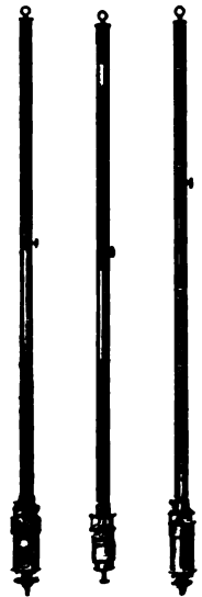
Fig. 718. Mercurial barometers of the cistern type.
