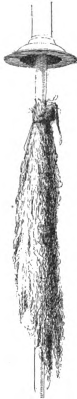
Fig. 576. Roots of an elm tree in a suction pipe in a dug well three feet in diameter.
