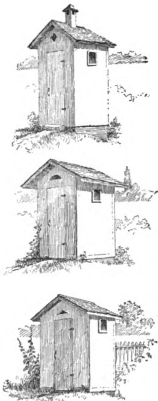
Fig. 278. A study in proportions. All these structures are of the same capacity and the doors are of the same size, but the buildings differ greatly in tastefulness.
