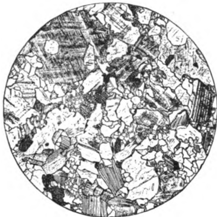
Fig. 451. Section of granite, magnified. The crystals are orthoclase, microcline, plagioclase, quartz, black mica or biotite, white mica or muscovite. (Merrill.)
