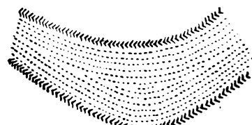
Fig. 550. Level terrace. Short rows in center of area.
