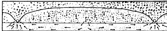
Fig. 570. Movements of water toward tile drains where heavy clay soils are underlaid with sand.
