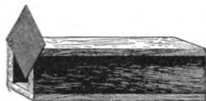
Fig. 600. Tube for diverting water to furrows.
