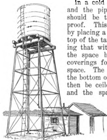
Fig. 413. The storage tank does away with the necessity for the continuous operation of the pump. The height of the tank varies with the purpose for which the water is to be used.
