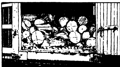
FIGURE 49.— Breakage and damage in a car of hampers loaded on their sides.
