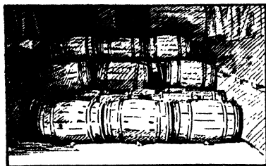
FIGURE 44.—Barrels loaded on their bilge crosswise of the car. Note that the barrels on the fourth layer should have been against the wall on the right.
