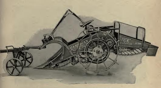
Fig. 26. Side view of a steel-nose potato-digger.
