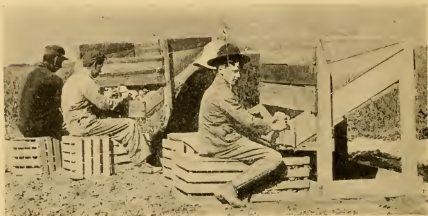
FIG. 25.—Seed-cutting hopper-boxes with stationary knives greatly facilitate the task of preparing the seed for planting. Courtesy of Daniel Dean, Nichols, N. Y.
