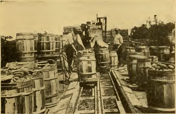
FIG. 88.—A handy labor-saving device for removing the barrels of sized potatoes from the sizer. Note small trucks operating on wooden tracks. By having two tracks with a truck on each there is no interruption in the operation of the sizer. On the G. W. Waller farm, Hastings, Fla.
