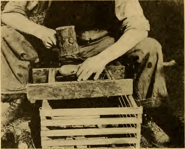
FIG. 27.—A set of adjustable knives fastened in a frame resting on a slat crate. A sharp blow from the wooden mallet forces the tuber through thereby dividing it as many times as there are blade sections covered.
