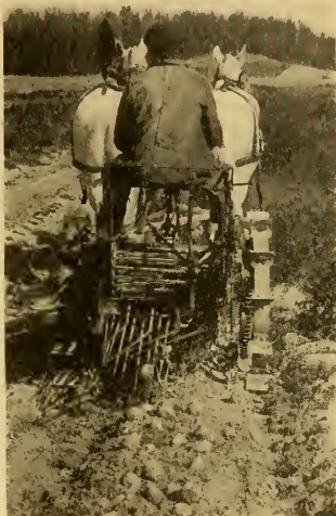
FIG. 80.—This elevator digger is being successfully operated by two horses without the aid of a gasoline engine. In this picture we have a good view of the vine and tuber separating rod rack.
