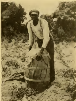
FIG. 100.—The hoop in place ready for nailing.
