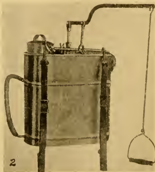
FIG. 192.—Knapsack Sprayer, carried on back of the operator. (Fights of the Farmer.)
