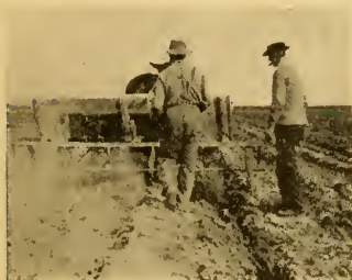
FIG. 12.—Applying fertilizer with a 3-row distributor.
