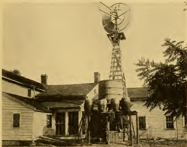
FIG. 186.—A spray mixing platform and equipment used by the U. S. Dept. of Agriculture at Honeoye Falls, N. Y. The only lifting necessary with this outfit was that involved in transferring the stock solutions to the mixing barrels.
