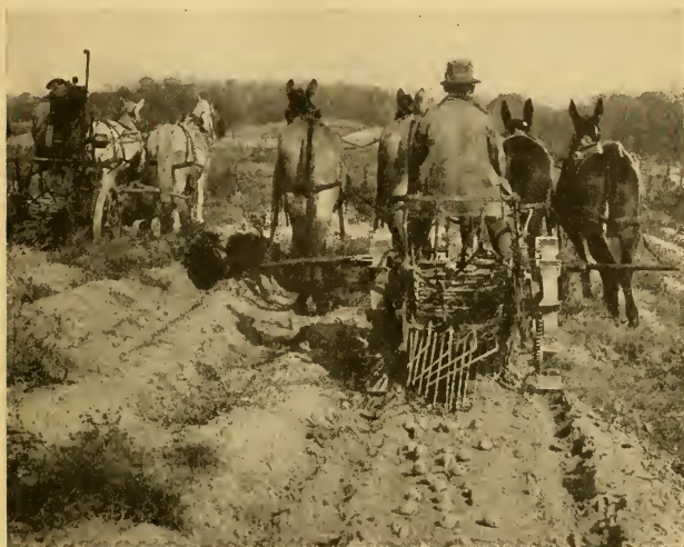
FIG. 82.—A four-mule team operates one digger while two horses and a gasoline engine operate the other.
