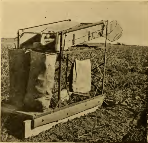
FIG. 89.—The western type of potato sizer mounted on sled runners to permit of hauling it with a horse or horses.
