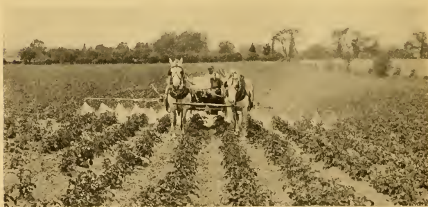
FIG. 197.—Spray outfit hauled by horses, pump operated by a gasoline engine mounted in front of spray tank. Courtesy of Bateman Mfg. Co.
