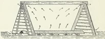
Frame of Potato House, Showing Ventilator in position.
