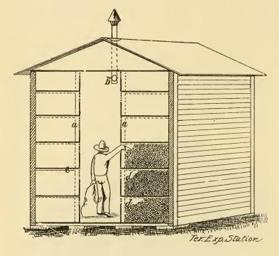
Fig 13—a. Posts which go up through the center from floor to ceiling. b, ventilator which may be opened in warm weather and closed in cold. c, Double wall. d, Potatoes stored in sand. e, Cross-pieces which run from posts to wall.
