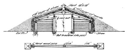
FIGURE 14.—Cross section of end elevation of potato-storage cellar at Carbondale, Colo., and top view of ventilated partition
