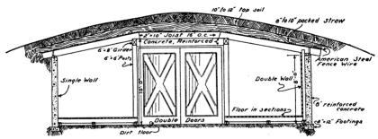
Figure 20.—Cross section of the end elevation of a potato-storage cellar at Jerome,  $\operatorname{Idaho}$
