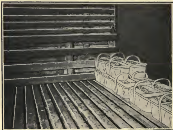
Racks Take up Surplus Space at End of Car and Prevent "Chucking."
