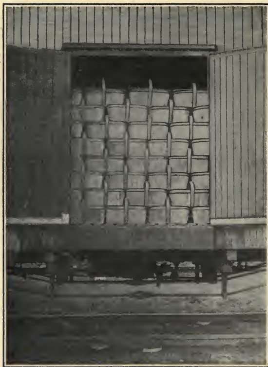
Car of Exact Width to Make Snug Load Without Placing Last Row Diagonally.
