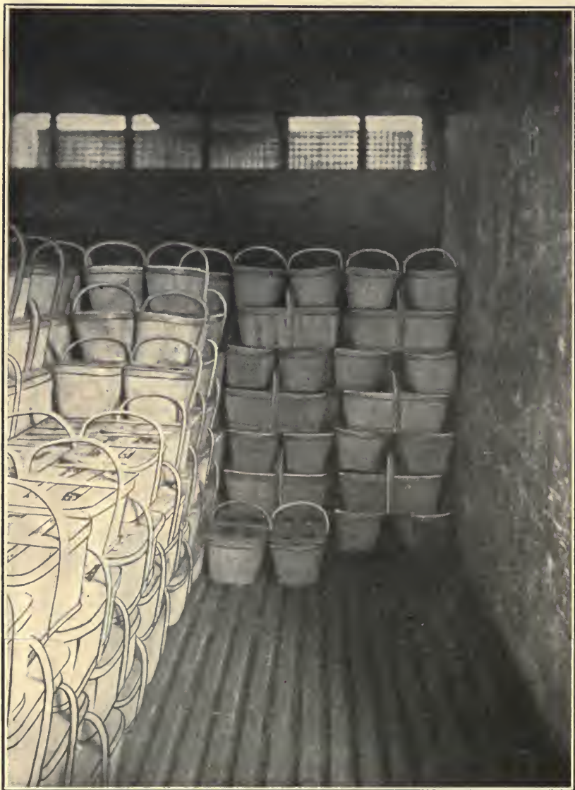
Loose Loads Like This Shift Badly in Transit and Cause Bad Breakage.
