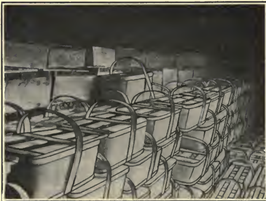
FIG. 26.—When it is absolutely necessary to load more than one kind of package in a car, the above method should be used with complete rows (only) of each kind of package, from end to end of car. Westfield, N. Y., Oct., 1917.
