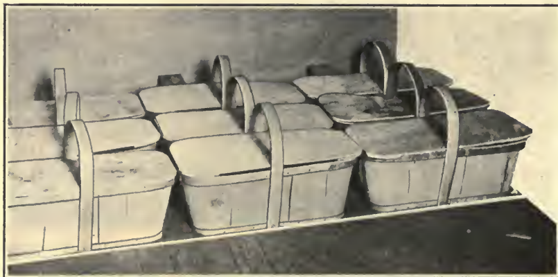
FIG. 30a.—Note that there are 4 inches of space between the car wall and the edge of the first basket.
