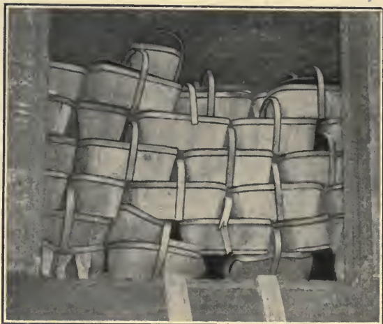
A Few Baskets Loaded Crosswise of the Car Caused this Breakage.
