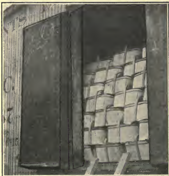
Load Shifted Because of Slack at Other Side of Car.
