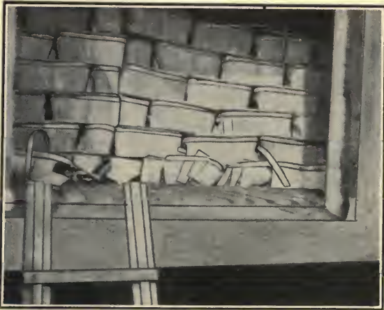
Breakage When Packages Catch on Car Floor.
