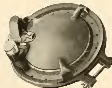
Bottom of hopper showing brush cut-off for Kafir corn and small seeds
