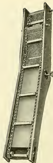
Husk conveyor or elevator. Note shelled-corn sieve at upper end
