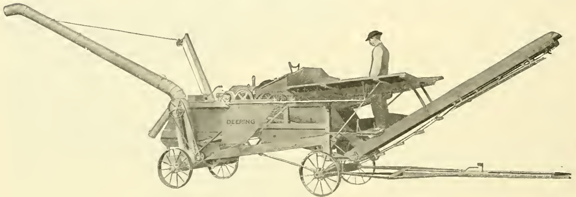
Right side of Deering 6-roll husker and shredder showing position of feeder
