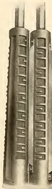
Snapping rolls. Note the V-shaped ridges on one roll which fit into the corresponding grooves on the opposite roll. There are 3 ridges and 3 grooves. A positive grip is thus secured as the rolls work toward each other.
