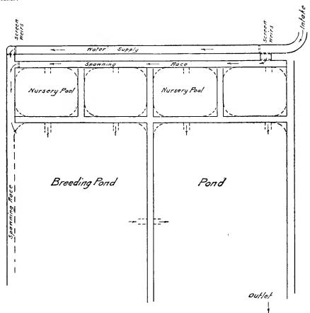
Fig. 1.-Plan of ponds and spawning race.
