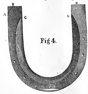
shoe, and come out on the foot surface in the flat part of the we'. and not partly in the flat and partly in the seating. It is a very bad plan to make them slant inward as most smiths do ; for in driving a nail, they have first to pitch the point inward, then turn it outward. driving it all the time with the
