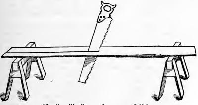
Fig. 3.-Rip Saw and manner of Using.
