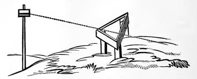
Fig. 83.—System of Leveling Small Plots of Ground.
