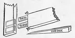
Fig. 56.—Mortises, Tenons and Wedge.
