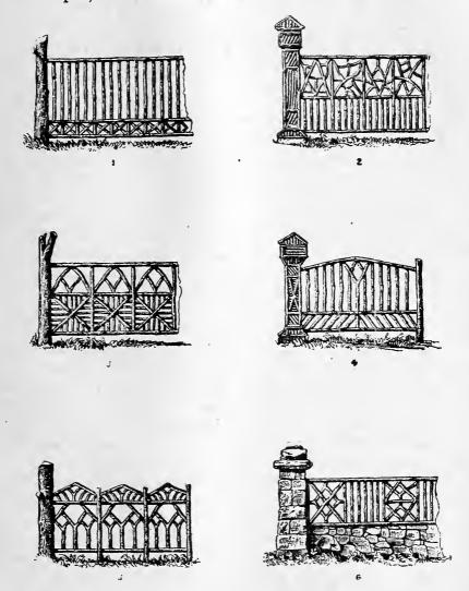
No. 6 has a very rough stone post, and a dwarf wall sixteen inches thick, coped with a rough blue-stone coping, and surmounted by rustic work secured by iron fastenings.
