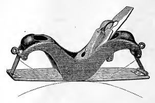
Fig. 35.—Patent Adjustable Circular Plane.
