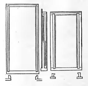
Fig. 85.—Door and Window Frames.
