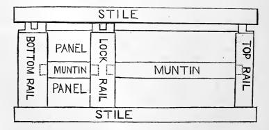
Fig. 54.—The Door Ready to Drive Together.
