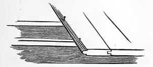
Fig. 84.—Specimen of Blind Nailing.
