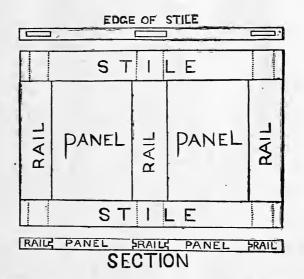
Fig. 2.— Carpenter's Tool Chest.— Sectional View.
