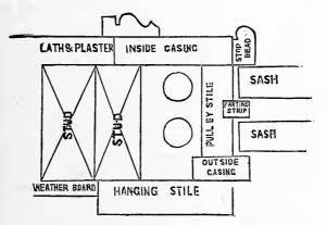
Fig. 90.—Construction of Box Window Frame.
