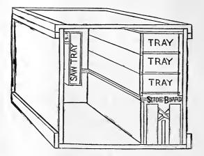
Fig. 1.— Carpenter's Tool Chest.
