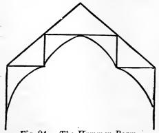
Fig. 94.—The Hammer Beam.
