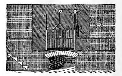
Fig. 12 is the front elevation of oven. 1, 1, 1 is iron work; 2, the sliding door; 7,7, the grooves in which it works; 3, the balance weight; 8,8, wheels on which the chain works; 4, aperture to admit gas; 5,5, level of oven bottom; 6, 6, 6, 6, the level of floor of bake shop; 9, valve-rod to clear the oven of steam; 10, valve-rod to drum; 11, valve-rod to chimney.
