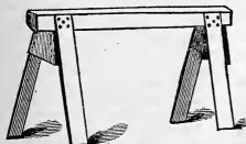
Fig. 46.—Carpenter's Saw Bench.
