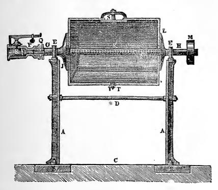
fluids carries too much water into the soap, the cause being the ready condensation of the exhaust steam. Live steam is applied directly to the grease and lye by various machines. One method is simply to introduce the steam by a cock into an open kettle containing the materials, and many of the best soaps are so made in England. Another method is with the closed vessel. A
