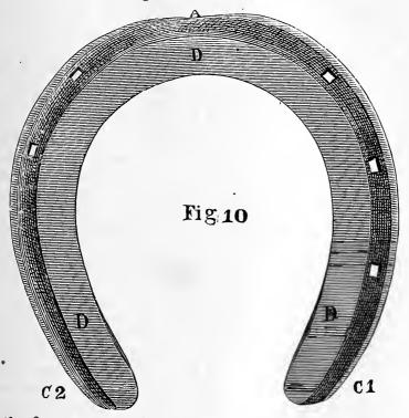
to the frog, so as to slant it from the ground upward away from the frog, but you must be careful not to make the ground surface of the web at the heels narrower in so doing; Fig. 9 shows the foot surface, and Fig. 10 the ground surface of a near fore shoe.
