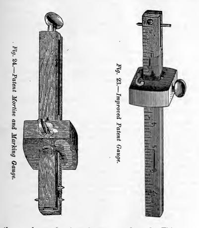
other can be regulated by the screw at the end. This gauge is used for marking out the mortises and tenons in framed work, as doors, or as in the chest lid shown in fig. 1, page 10. The mortises are cut out with chisels, and the tenons set in the bench screw, and cut down with the rip saw. There are also panel gauges for marking the width of broad panels, and cutting gauges, in which the points are knives which make a cut of a quarter or half an inch in depth.
