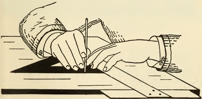
Fig. 10—Correct Manner of Holding a Ruling Pen.
