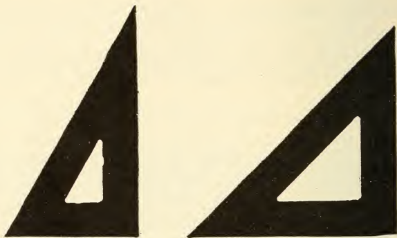
Fig. 13—60 and 45 Degree Triangles.
