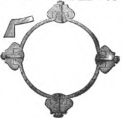
Built Iron Column.
