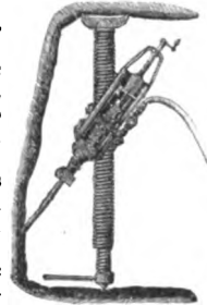
Drill Mounted for Shaft Work.
