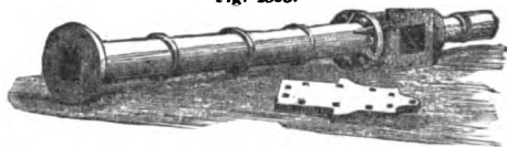
Working Barrel of Cornish Pump.
