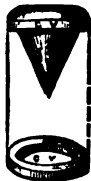
Fig. 2126 shows the position of a retaining valve placed near to the air-vessel of a heavy pumping engine to prevent any water leaking back through the pumps when the engine is stopped. It also admits of the pumps being examined without emptying the up-take.
