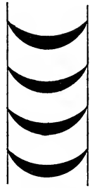
FIG. 157. — Arrangement of blade thickness to give uniform passage width.
