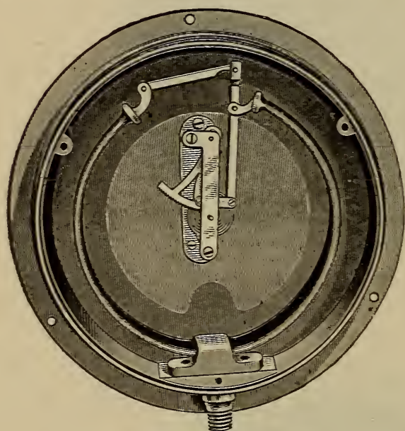
FIGURE 182 SECTIONAL VIEW AMERICAN PRESSURE GAUGE
