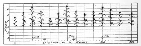
Fig. 9. Diagram Showing the Effects of Drainage Upon the Height of Corn at Hanford, Cerro Gordo County, Iowa, October, 1910.
