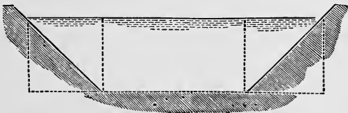
Fig. 129.—PLAN OF MEASURING A CROSS-SECTION.
