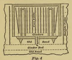
The success of this method depends largely on the sand under and around the pattern being evenly tempered, and sufficiently porous to permit the gases to circulate freely. See Fig. 6.
