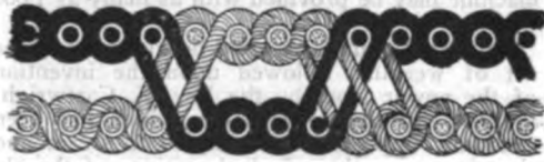
FIG. 14.—Sectional Diagram of one of the many methods of weaving double cloth on two sets of warp.
