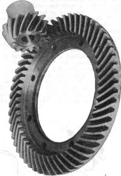
FIG. 17.— Spiral bevel gear wheel with driving-pinion.
