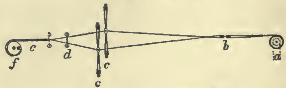
FIG. 26.—Section of Plain Web in Process of Weaving on the Loom. a, The warp beam. d, The reed in position for picking, and also for beating-up. b, The lease rods by which the warp is divided and crossed. c, Woven cloth. c, c, Two pairs of shafts containing healds. f, The cloth beam.
