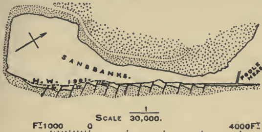
FIG. 13.—Groyne for Protecting the Sand-banks enclosing Poole Harbour.
