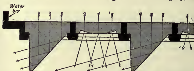
FIG. 2.—Section through Prism Pavement Light, the direction of light rays being indicated by arrows.
