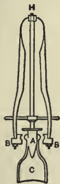
FIG. 18.—Tool for moulding the inside and outside of the neck of a bottle.
