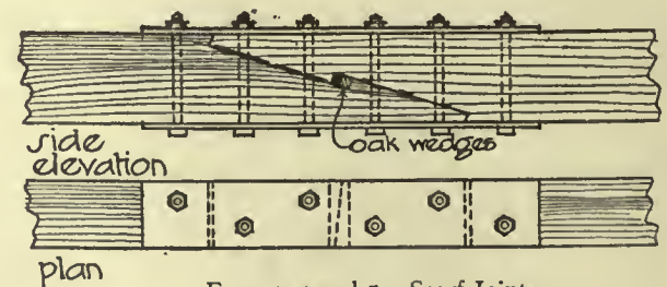
FIGS. 3, 4 and 5.—Scarf Joints.
