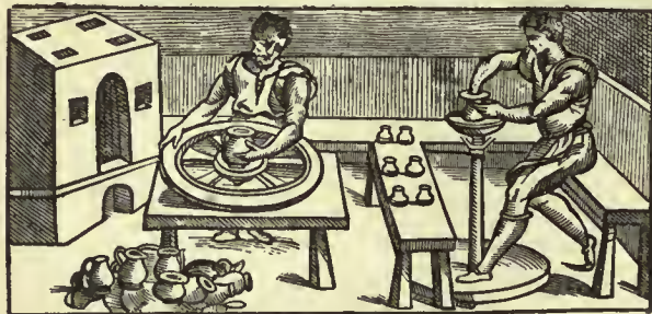
FIG. 5.—Two forms of Italian potter's wheels, about 1540.
