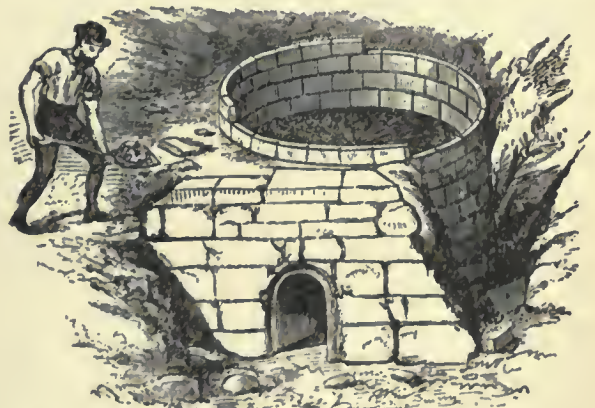
FIG. 4.—Roman kiln found at Castor. The low arch is for the insertion of the fuel; the pots rested on the perforated floor, made of clay slabs; the top of the kiln is missing,—it was probably a dome.
