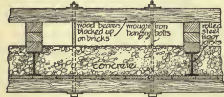
FIG. 20.—Method of supporting Centering for Concrete.
