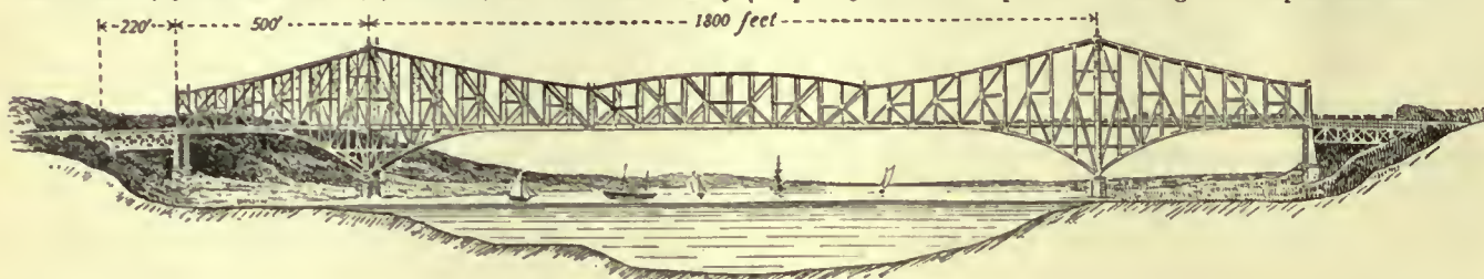
FIG. 25.—Quebec Bridge (original design).
