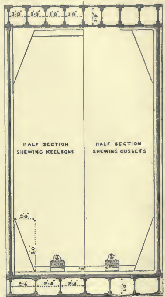
FIG. 17.—Britannia Bridge (Cross Section of Tubular Girder).
