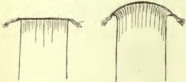
FIG. 10.—Section of back of book sewn on bands. FIG. 11.—Section of same book after it has passed through the machine for rounding and backing.
