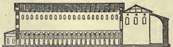
FIG. 13.—Section of the Basilica of St Paul, Rome.
