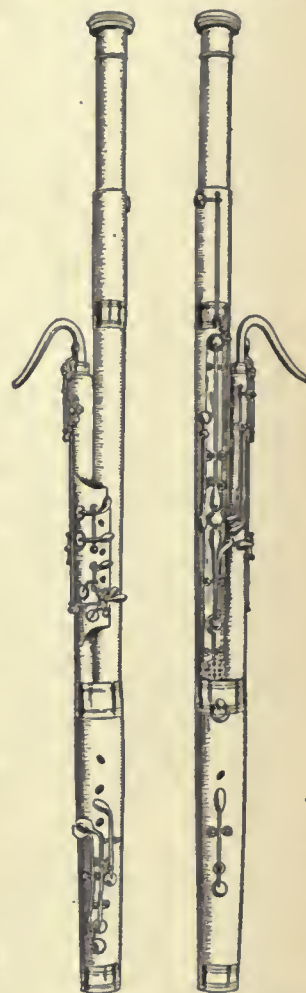
Front view. Back view. FIG. 1.—Bassoon with 17 keys. Savary Model. (Rudall, Carte & Co.)
