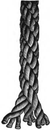
Drilling cable, hawser laid
