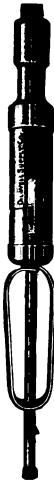
Showing position of perforators when the tool is being lowered into casing.
