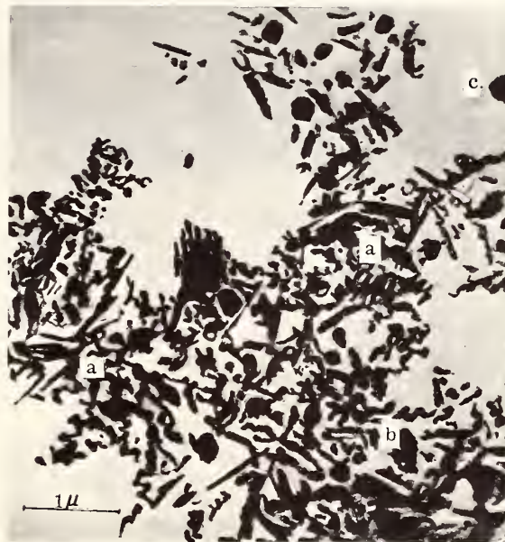
Fig. 7. The form of particles smaller than 0.001\text{ mm} in Lower Cambrian clays consisting of hydromica (a) and sericite (b) with admixtures of kaolinite (c).
