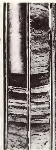
Fig. 42. Soil sample from a vibrodrilled hole. The photograph shows that the fine bedding is undisturbed.
