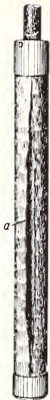
Fig. 19. Water (a) flowing to the surface of the vent in the sectional barrel.
