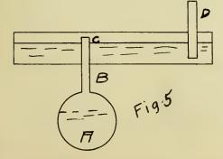
containing boiling water, with a pipe P reaching nearly to the bottom. As the steam accumulates it presses on the surface of the water, and will force it in a jet through the pipe,
