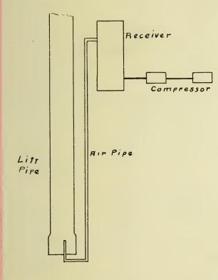
The accompaning figure illustrates a compressor, receiver air and lift pipe as usually operated in deep wells, in which the pressure in the air pipe must be greater than the hydrostatic pressure of the water at the bottom of the pipe, and in quantities sufficient to make the ascending column of air and water in the flow pipe lighter in its total height than
