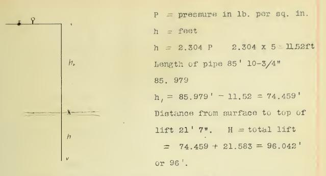
If x = the number of cubic feet of water pumped, 62.5X the number of pounds pumped. The number of foot pounds of work done is equal to the total weight in pounds times the lift in feet. The number of pounds of steam taken to do this work is also known, therefore the duty or foot pounds of work done per 1000 pounds of steam can be determined.
