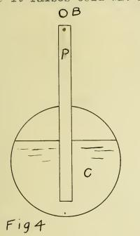
has a neck or tube B, through which the steam passes to the upper part of the cistern C, and, pressing on the surface of the water it contains forces the water upward and out of the pipe D. This principle was used in various contrivances and for a long while it was the most advanced form of water elevator..
