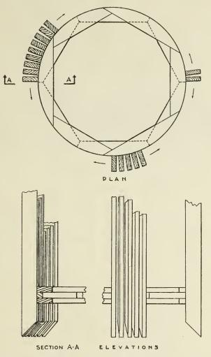
Fig. 18.—Special cylindrical wood cribbing with planking mounted on edge, facing outward, to make slotted wall for entrance of water.
