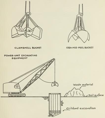
Fig. 6.—Power equipment for excavating.
