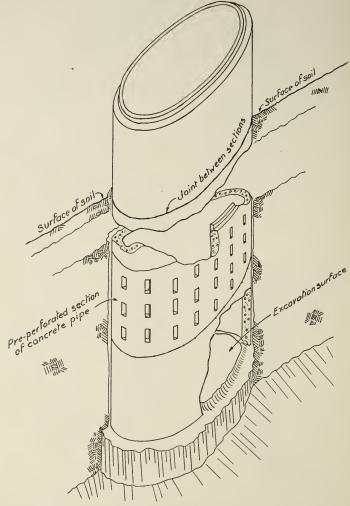
Fig. 19.—Large-diameter concrete pipe used as well lining, including perforated sections.
