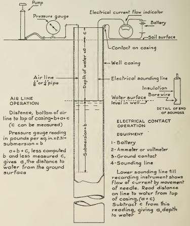
Fig. 26.—Devices for measuring depth to water.
