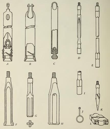
Fig. 9.—Cable tools: A, suction or sand bucket; B, scow or bailer; C, dart-valve bailer; D, jars; E, drill stem; F, standard bit; G, star bit; H, heavy-duty bit (spudder type); I, rope-sub; J, bit gauge; K, swage; L, drive clamps.
