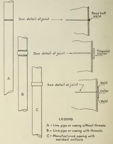
Fig. 22.—Detail of three types of casing and the corresponding joints.
