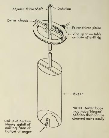
Fig. 11.—Power-driven auger, with portion of driving mechanism.
