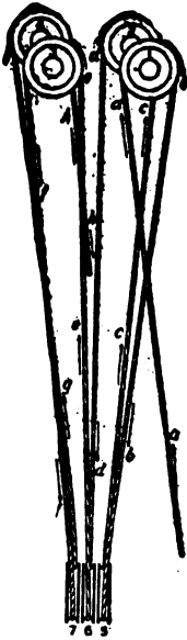
Fig. 163 Method of stringing casing blocks
