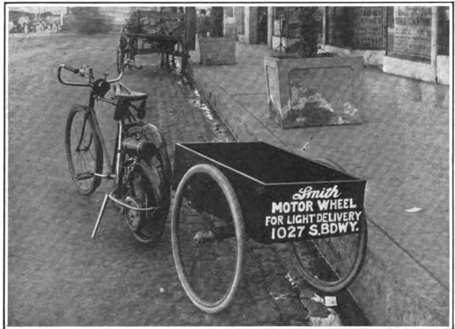
The Outfit Is in Use in Los Angeles and Has Given Excellent Results; the Trailer Is Attached by a Swivel Connection to the Bicycle
