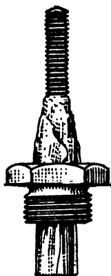
The shaft wound with India mica by hand, showing bushing forced on.
