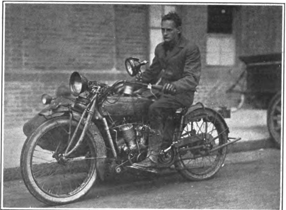
Jack Neis and the Indian on Which He Displayed New Splitdorf Generator and Separate Ignition System for Atlantic City Trade Visitors
