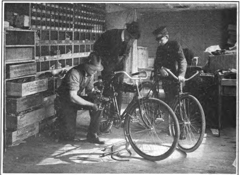
Photograph Shows a Bicycle in the Process of Being Motorized by Attaching the Popular Cyclemotor, the Little Rochester-Made Motor Plant
