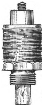
Loose mica washers—before being compressed and turned down and shaped.
