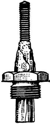
First Winding of Mica—with bushing forced on.
