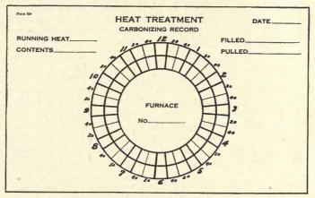
Blank for recording Furnace Temperatures
