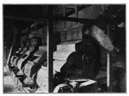
FIGURE 20.-Small-drum cleaning feeders, with mechanical or belt distribution system.
