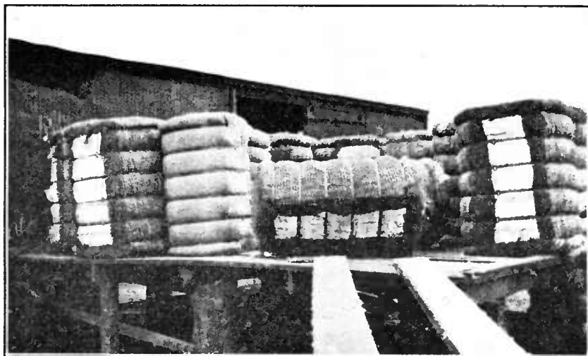
FIG. 20.—Railroad platform full of uncompressed cotton ready for loading on freight car, to be shipped to the compress
